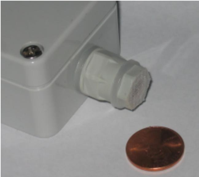
The SHT75PG here is mounted on a sealed polycarbonate enclosure. The sensor element itself is protected under a membrane permeable to water vapor. The enclosure can be drilled 7/16" and tapped PG7, or the enclosure can be drilled 1/2" and a PG7 nut (included) installed on the inside. Inside the enclosure can be a data logger or transition wiring to a cable.
