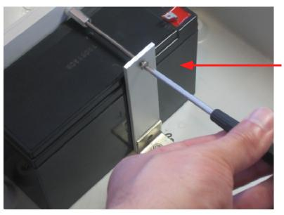
screw the #6 2-1/4" machine screw into the #6 standoff, until the battery is held firmly in place.
