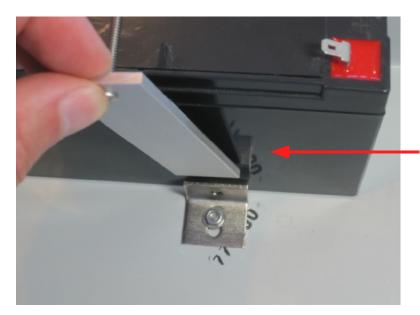
place the 1/8" aluminum bar between the corner bracket and battery (the black, soft side of the bar faces the battery).
