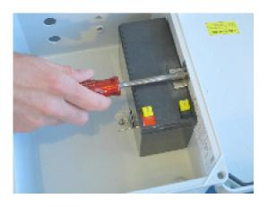
2) Loosen the #8 nut that holds the bottom of the battery in place. Once the nut is loosened, slide the metal bracket away from the battery.
