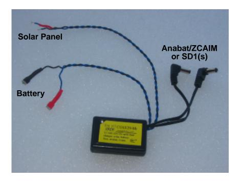
Battery charger, CG1129BH. -- for 12 volt sealed Pb-acid battery.
