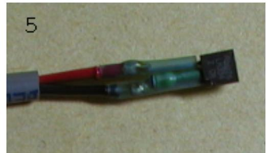
Photos 2 & 3. The center leg of the LM334 and one lead of the resistor are trimmed to 1/8" long. The resistor is soldered to the center leg and covered with the short length of shrink tubing. The simple jig in photo 2 helps to align the parts for soldering.
