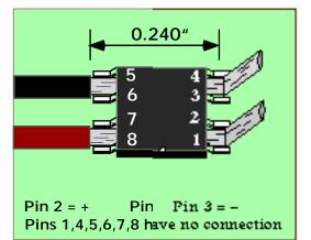
Only 2 pins on the 8-pin package are connected.
