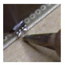
Solder pins 1 and 2 to the red (+) wire, and solder pins 3 and 4 to the black (-) wire.
