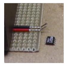
Strip wires back 3/8" and tin. Bend wires up 0.240" out from the insulation.
