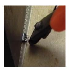
Clamp the chip, trim the wires. Or you could trim the wires before placing the chip.
