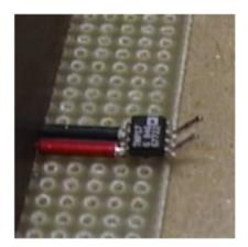
Set the chip on top of the bent wires.
