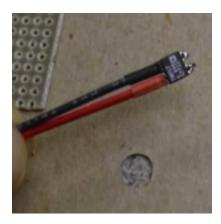
Shrink tubing over individual wires is optional. Shrink tubing can hook over pins 5,6 and 7,8 for added mechanical strength.
